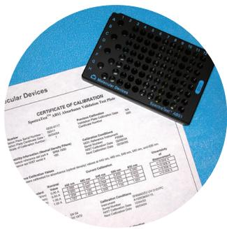
**Absorbance detector validation.** The SpectraTest ABS1 Absorbance Plate is used to validate optical performance of SpectraMax, FlexStation 3, and VersaMax microplate readers.
