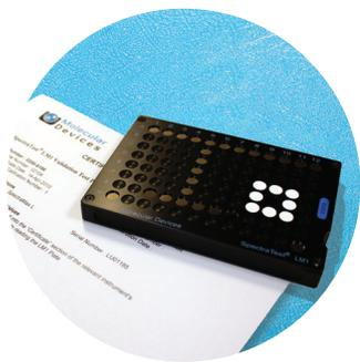
**Luminescence detector validation.** The SpectraTest LM1 Luminescence Plate is used to validate optical performance of SpectraMax i3, i3x, M3, M4, M5, M5e, L, and FlexStation 3 microplate readers.
