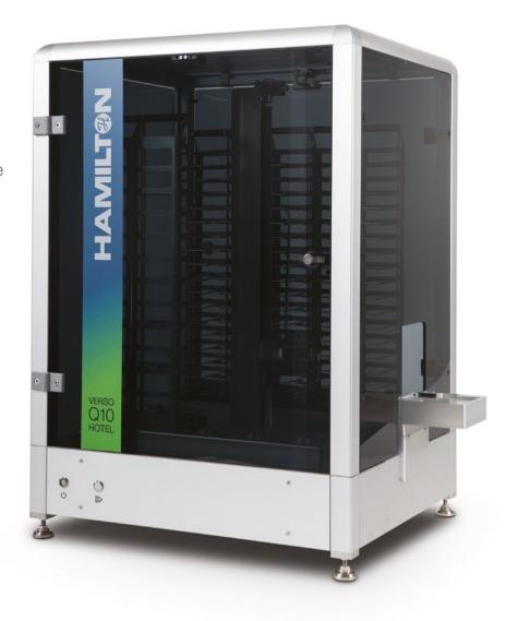
Advanced software uses the latest web-based technologies, so that system management and inventory status may be accessed remotely through a computer or mobile device. Standardization in Laboratory Automation (SiLA) 2 compliant interface ensures that Verso Q10 Hotel is future ready. Additionally, dedicated drivers are available for Hamilton's powerful automated liquid handlers.
