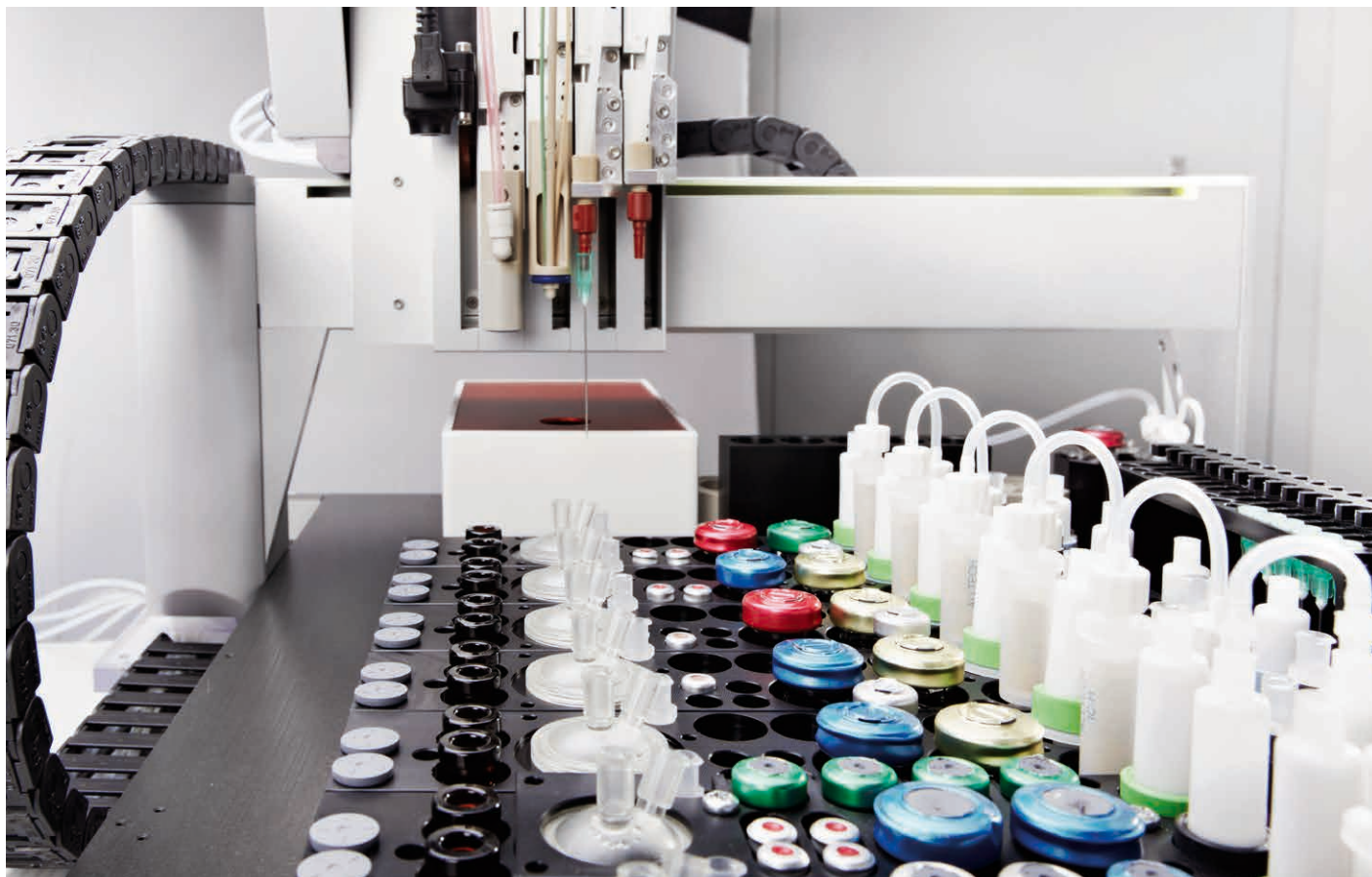
Work plate of the BioSyntheSizer, a multi-synthesis radiopharmaceutical robot that is also suitable for other chemical syntheses
