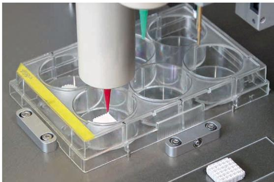
The new **multi-Z-drives** can print different materials at various pressures and temperatures, without exchanging cartridges. Many additional tools can be mounted.
