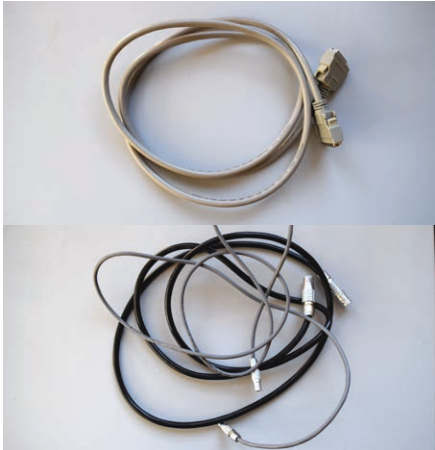
Cables for BS3.1 (top: data cable, can be longer), to be mounted between main unit and F-Box
