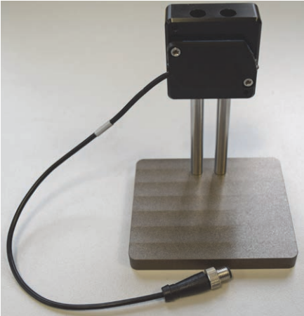
Liquid level sensor built into the PCV holder (the latter without Velcro fastener)
