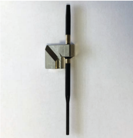
A051-184 Dosage capillary (“passive” tip) for bulk volumes; it is no disposable and has to be washed between different samples
