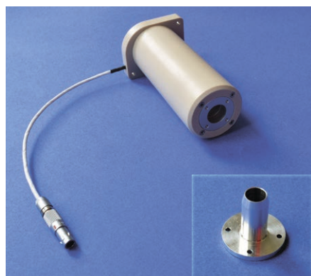
A051-210 Holder for 10 ml cartridges with heater and cable; for up to 120 °C. Inset: heat shield for metal nozzles (A051-240), which is connected to the bottom of the heatable holder via four small screws.
