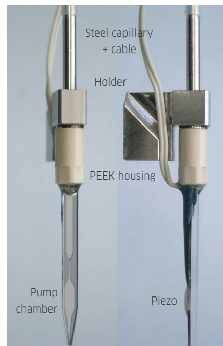
A070-401 Nano-Tip, front and side view; silicon and glass layers and the silicone cover on the piezo actuator can be seen (overall size of Pico-Tip identical)
