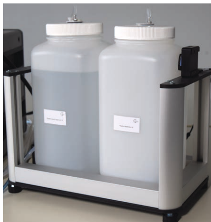
A051-845, -850 Wide-mouth reservoirs (complete) for system liquid and waste, 4 litres, in their rack (rack not included)
