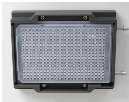
Cooled microtitre plate holder for one source MTP (this one is from the Nano-Plotter; the BS3.1 version is different)
