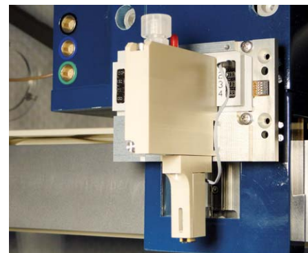
For bulk dispensing of a larger number of smallest drops (from 10 Pikolitres) a reservoir (3 Millilitres) is available for the piezoelectric tips.
