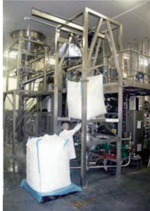
FIBC station with tilting table, lumpbreaker and Jet-Mixer
