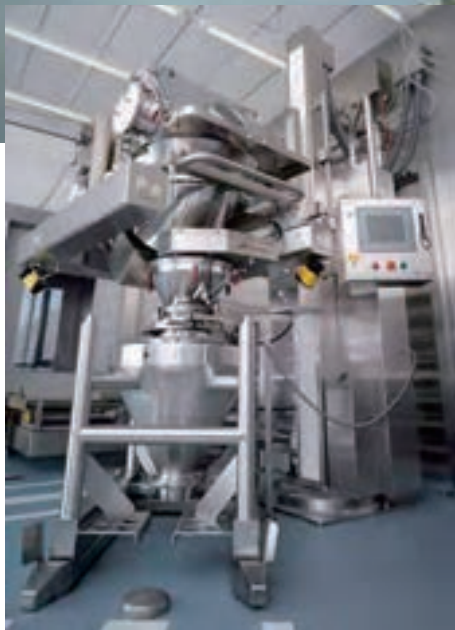
Multi-Dosimat mounted on the lifting column to dose into IBC
