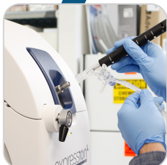
iASAP: Direct Analysis of Air-Sensitive Compounds
