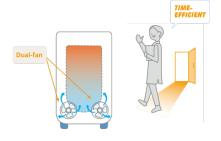
The SX-E series Autoclaves are standard-equipped with a dual-fan cooling system, shortening overall operation time.
