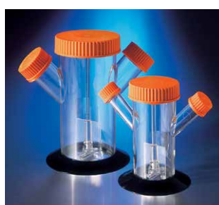
Disposable spinner flasks (Cat. Nos. 3152 and 3153)
